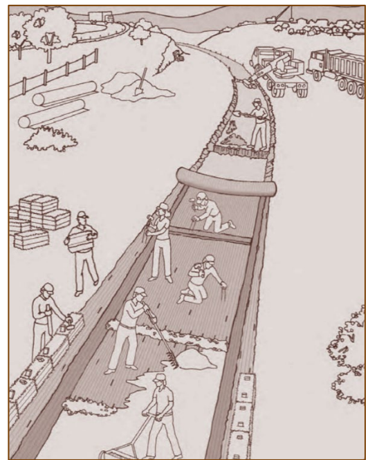
Figure 5- 14 Example of TRM Channel Application
