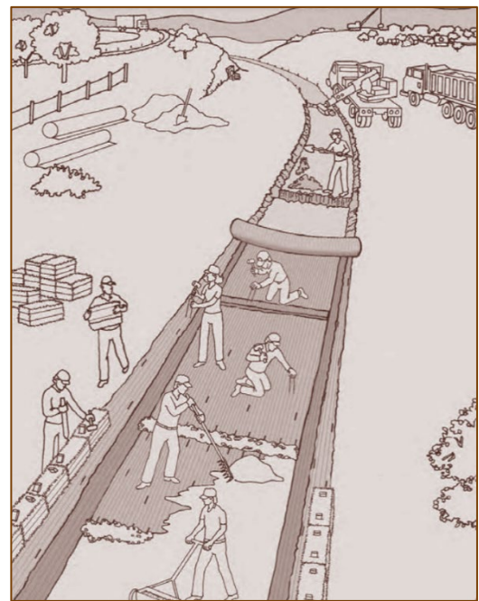
Figure 5- 14 Example of TRM Channel Application
