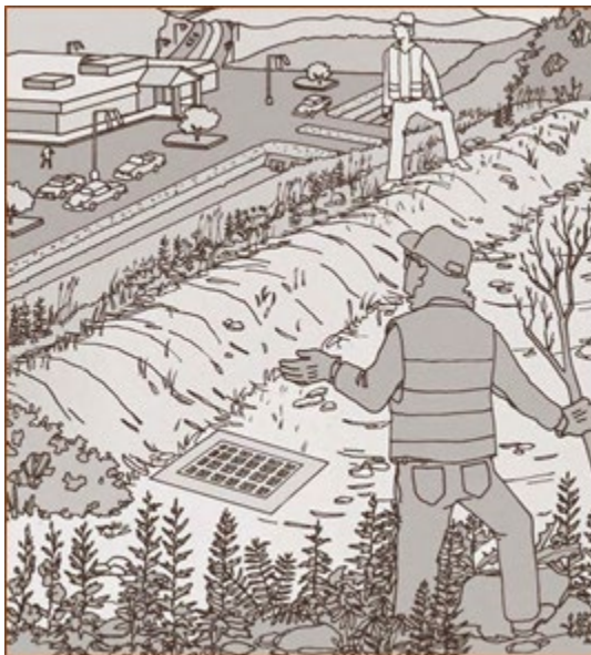
Figure 5- 52. Illustration of Permanent Diversion Intercepting Overland Flow
