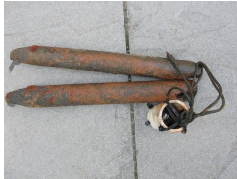
Examples of loggers secured within PVC tube using zip ties and then attached to a heavy metal weight. Shown is a railroad tie (left) and old window weights (right).
