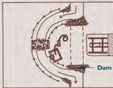
Figure 4-5B Diversion Channel Crossing Sequence
