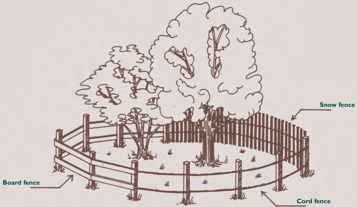
Correct methods of fencing tree protection zones
