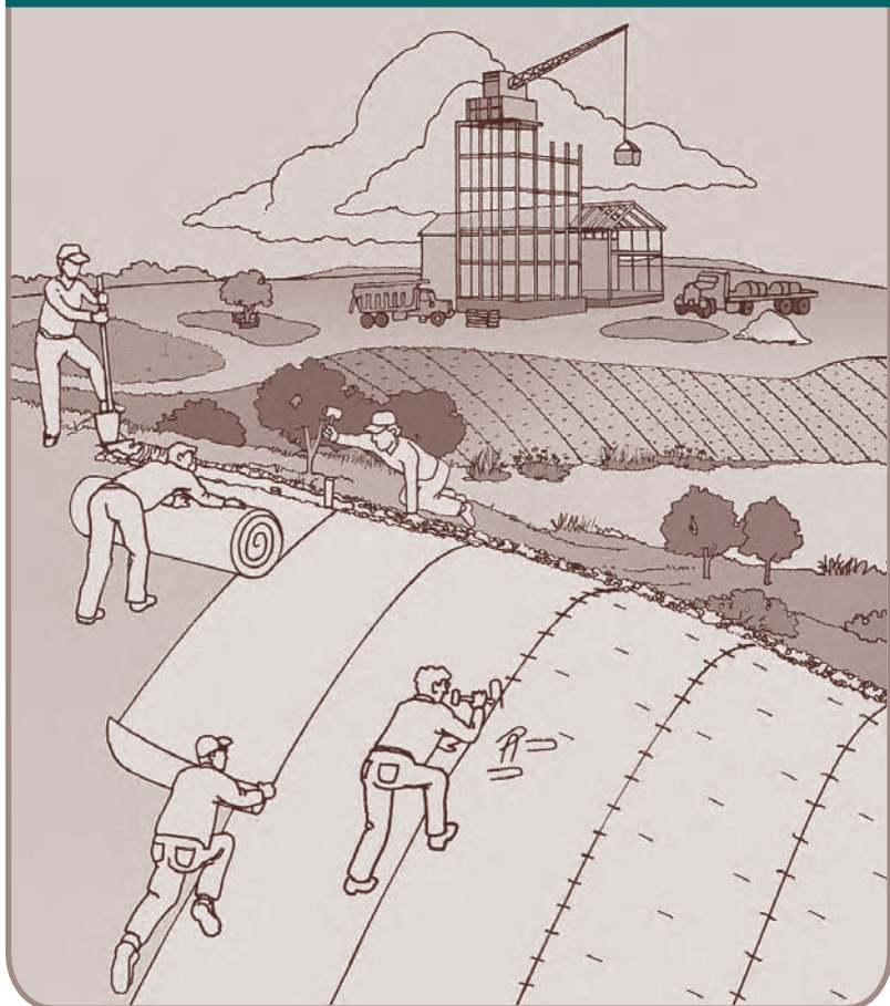
Figure ECB-1 Example of Temporary Erosion Control Blanket Installation
