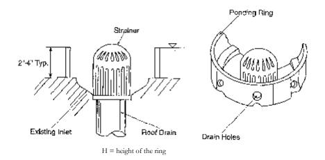
Figure 5.26 - Roof ponding rings. Source: Adapted from Tourbier, 1974.
