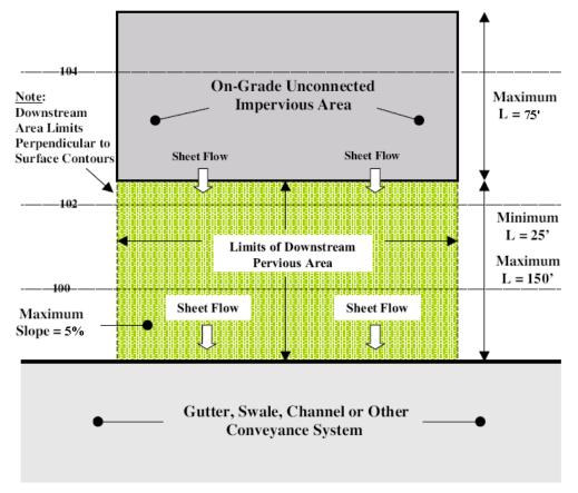
Figure 5.19 – Standards for disconnecting impervious surface via sheet flow. Source: Adapted from New Jersey Department of Environmental Protection, 2004.
