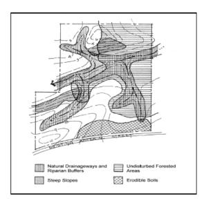
Figure 5.2 shows a site map with undisturbed natural areas delineated.
