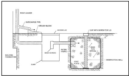
Figure 5.29 – Schematic of a drywell with optional sump to facilitate cleanout. Source: Adapted from New York, 2001.
