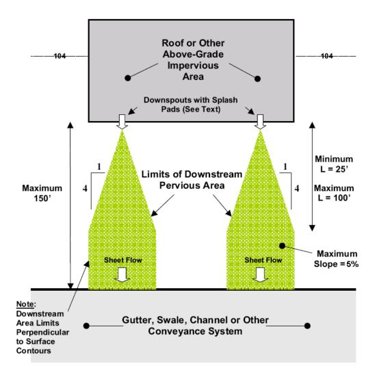
Figure 5.20 – Standards for disconnecting impervious surface via downspouts. Source: Adapted from New Jersey Department of Environmental Protection, 2004.
