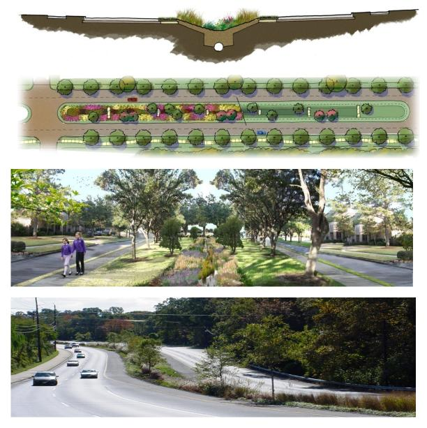
Figure 4.10 – Examples of center median detention/infiltration/filtration systems.
