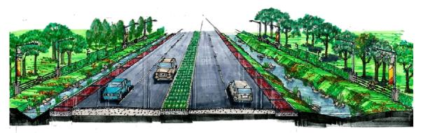
Figure 4.11 - Shoulder Treatment Systems using detention and filtration design.
