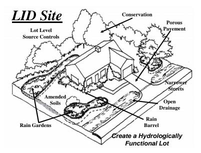
Figure 4.1 – Schematic of engineered practices.
