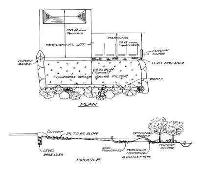
Figure 5.22 – Drawing of a vegetative filter strip. Source: Adapted from Atlanta Regional Commission, 2001.
