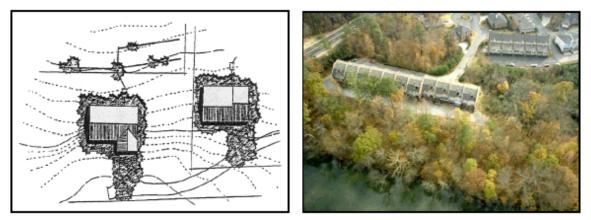
Figure 5.1 - Reduced limits of disturbance minimize water quality impacts. Source: Adapted from Atlanta Regional Commission, 2001.
