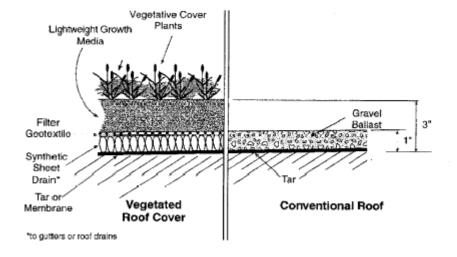
Figure 5.27 - Example Vegetated Rooftop Cross-section
