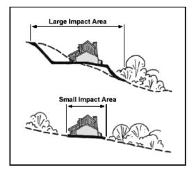
Figure 5.6 – Building on flatter slopes reduces the impact of development. Source: Adapted from Atlanta Regional Commission, 2001.
