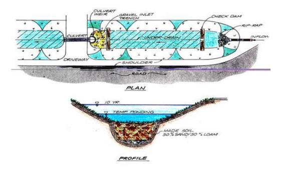
Figure 4.8 - Swale design to enhance its ability to filter and infiltrate runoff.
