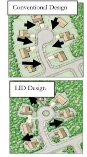
Figure 3.6 - conventional approach of draining runoff to the streets vs. a LID design using site fingerprinting.
