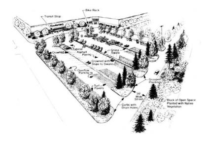
Figure 5.16 – Parking lot with islands attractively integrated. Source: Adapted from Connecticut, 2004.
