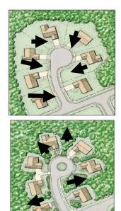
Figure 2.2 - conventional approach of draining runoff to the streets vs. a LID design using site fingerprinting.
