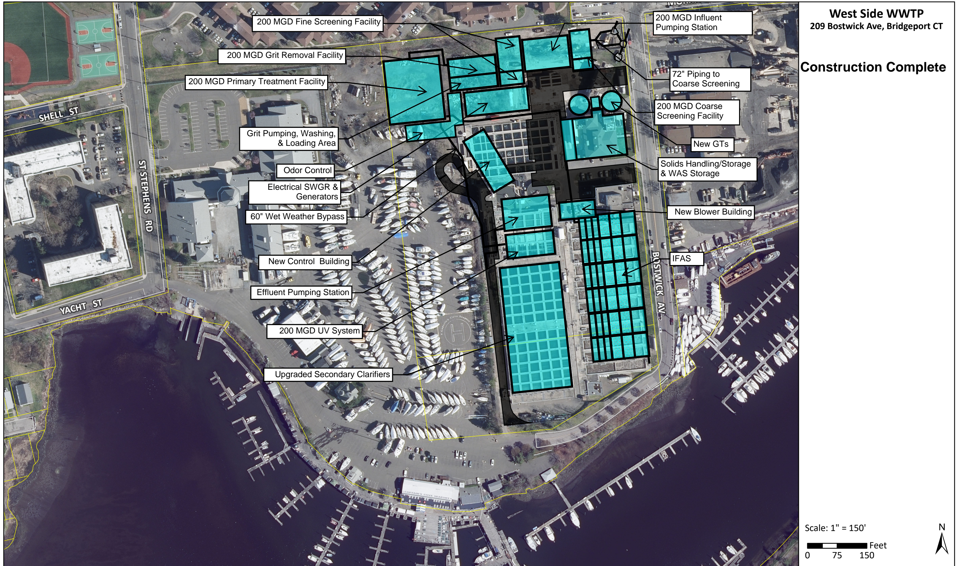
Figure 9.1-81 West Side WWTP MOPO Sequence - Construction Complete
