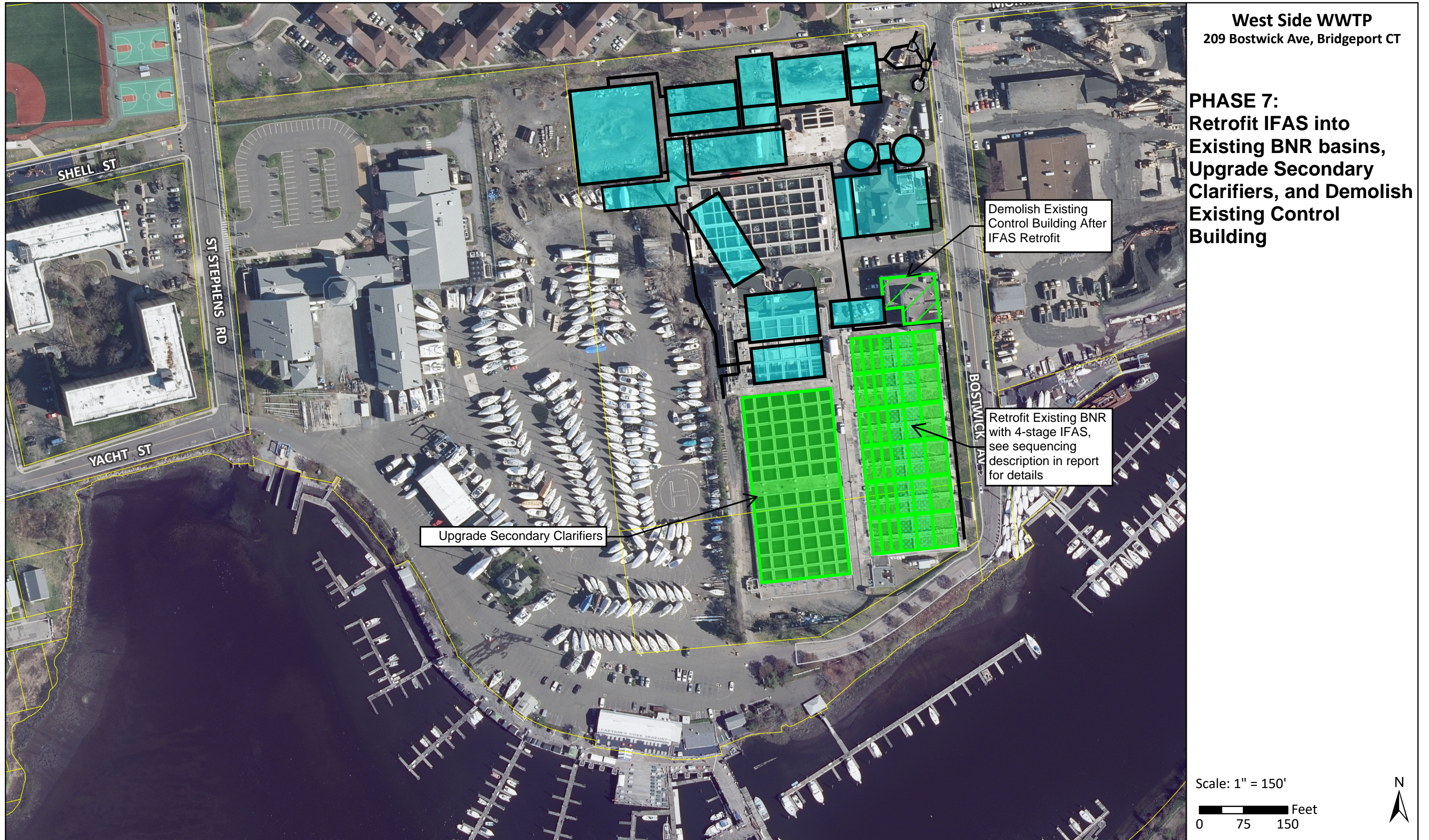
Figure 9.1-8G West Side WWTP MOPO Sequence - Phase 7
