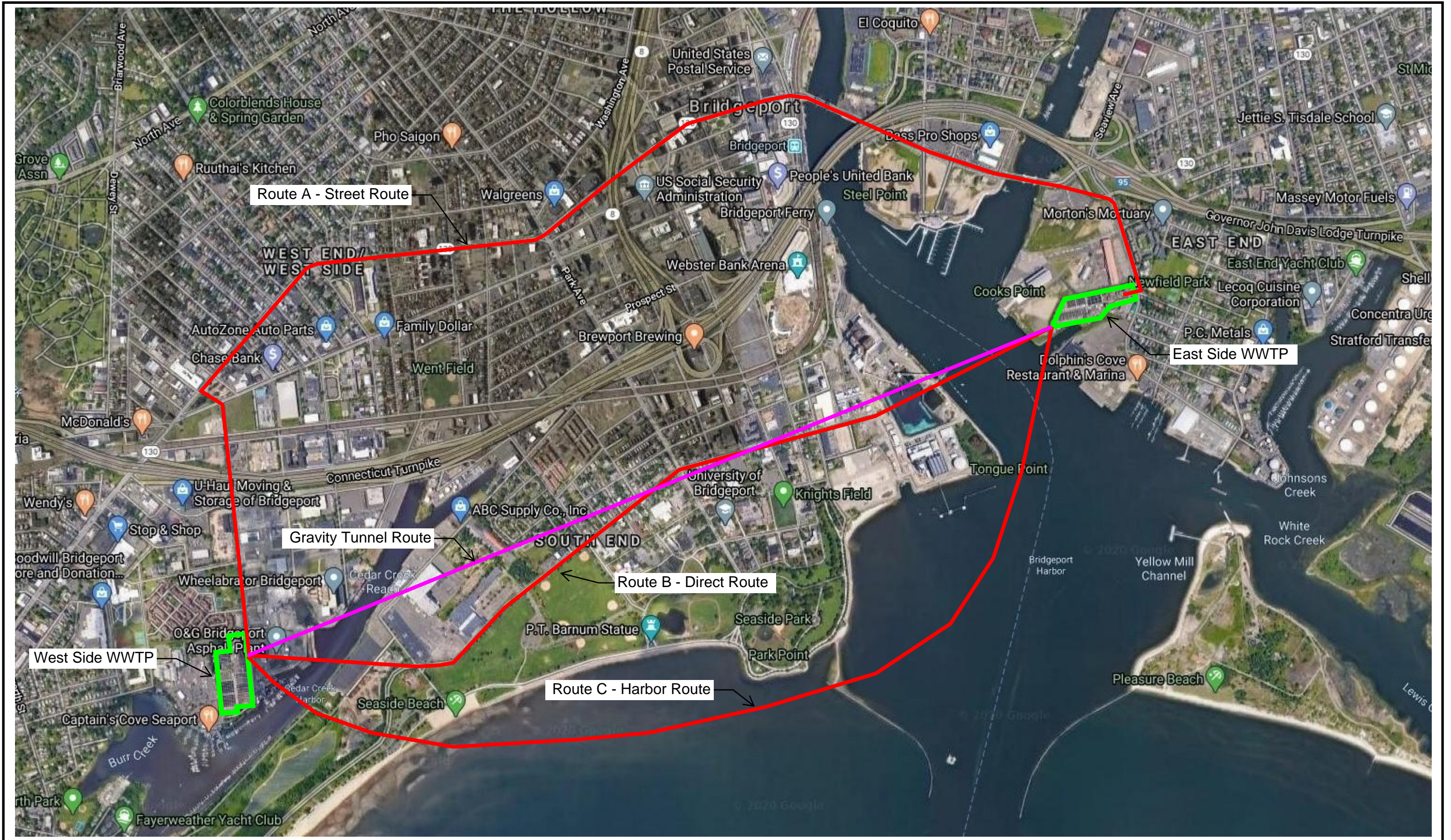
Figure 6.3-1 Pipe Routes Between West & East WWTPs
