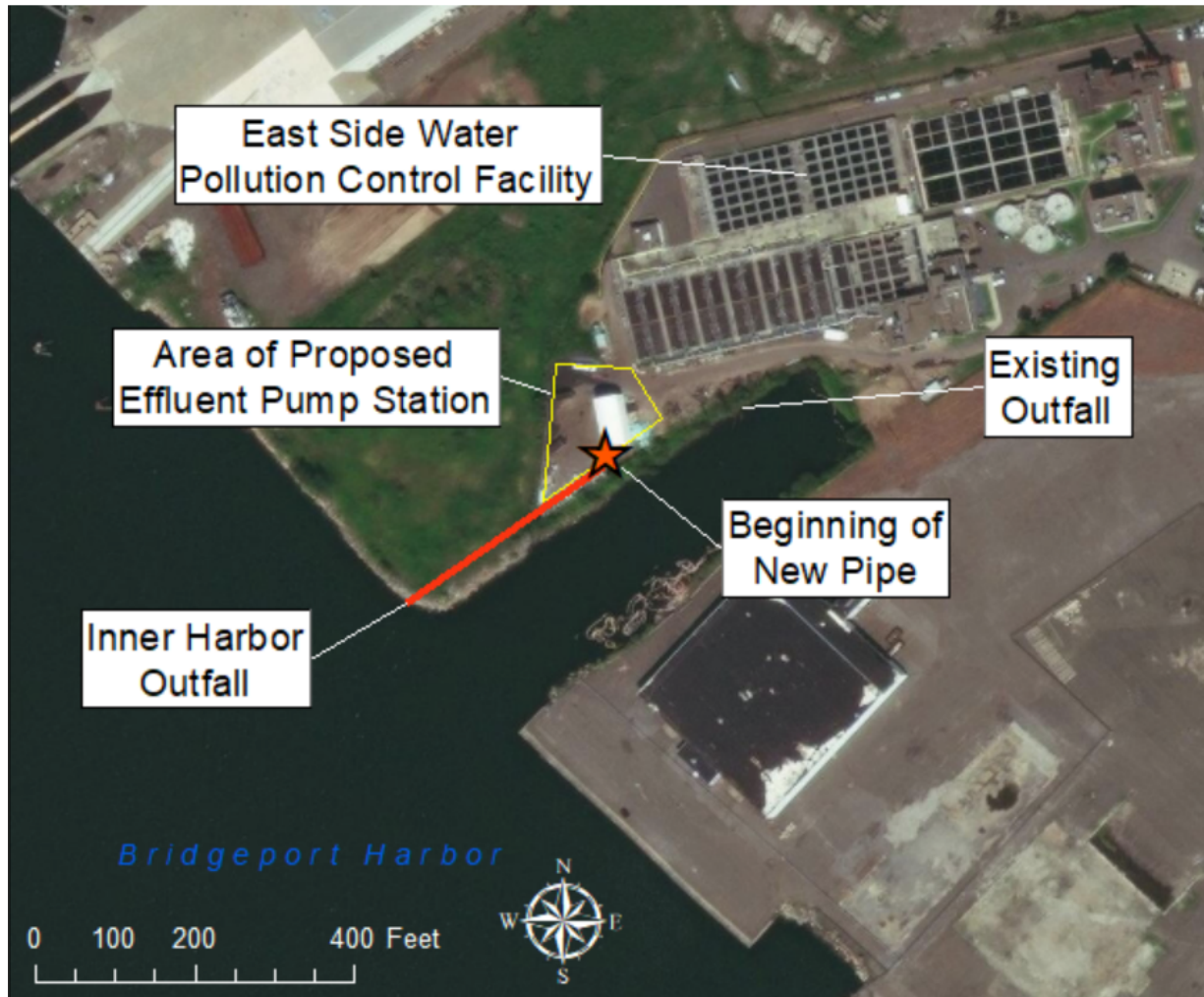
Figure 6.10-5 East Side Plant with Existing Outfall and Alternative Outfall Location in the Inner Harbor
