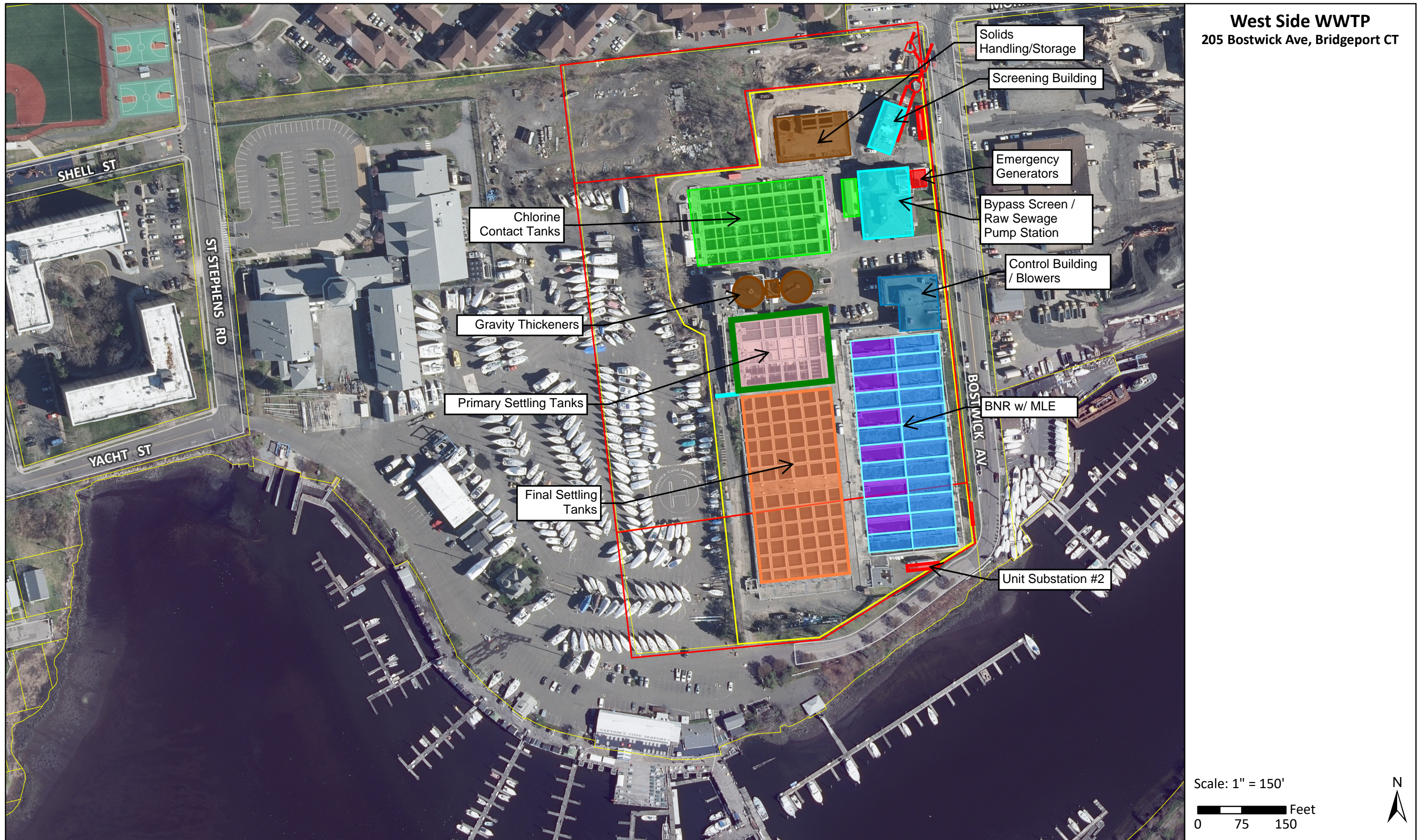
Figure 4.2-2 Existing Conditions - West Side WWTP
