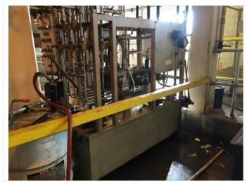
5. 90 Gallon hydraulic oil tank for screen unit.
