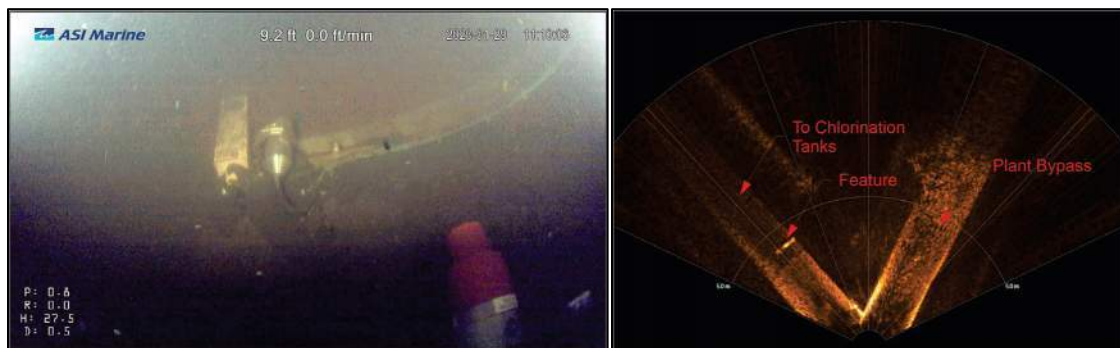
Figure 12: Image of sensor at 9 feet upstream (left); Sonar image looking down conduits toward CCT and plant bypass from manhole 1 junction (right)
