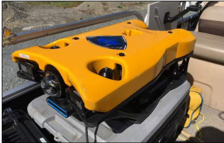
Figure 3: MSS Defender configured with camera, sonar, and profiler
