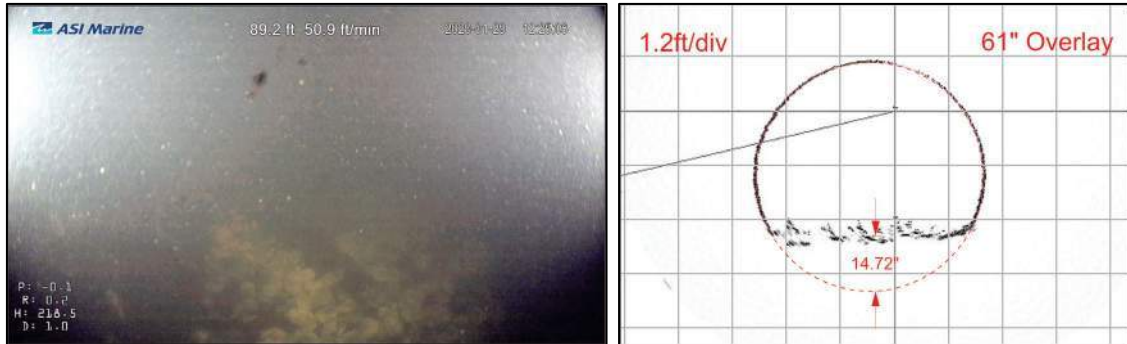
Figure 14: Image of sediment and rock debris at 89.2 feet (left); Profile image of debris at 145 feet (right)
