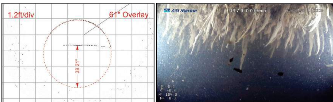
Figure 13: Profile image at 16.7 feet in bypass (left); Image of crown at 16.7 feet in bypass (right)
