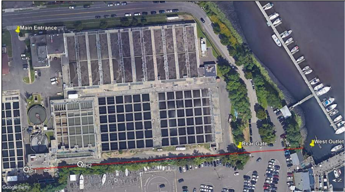
Figure 2: Overview of approximate west outfall piping routes
