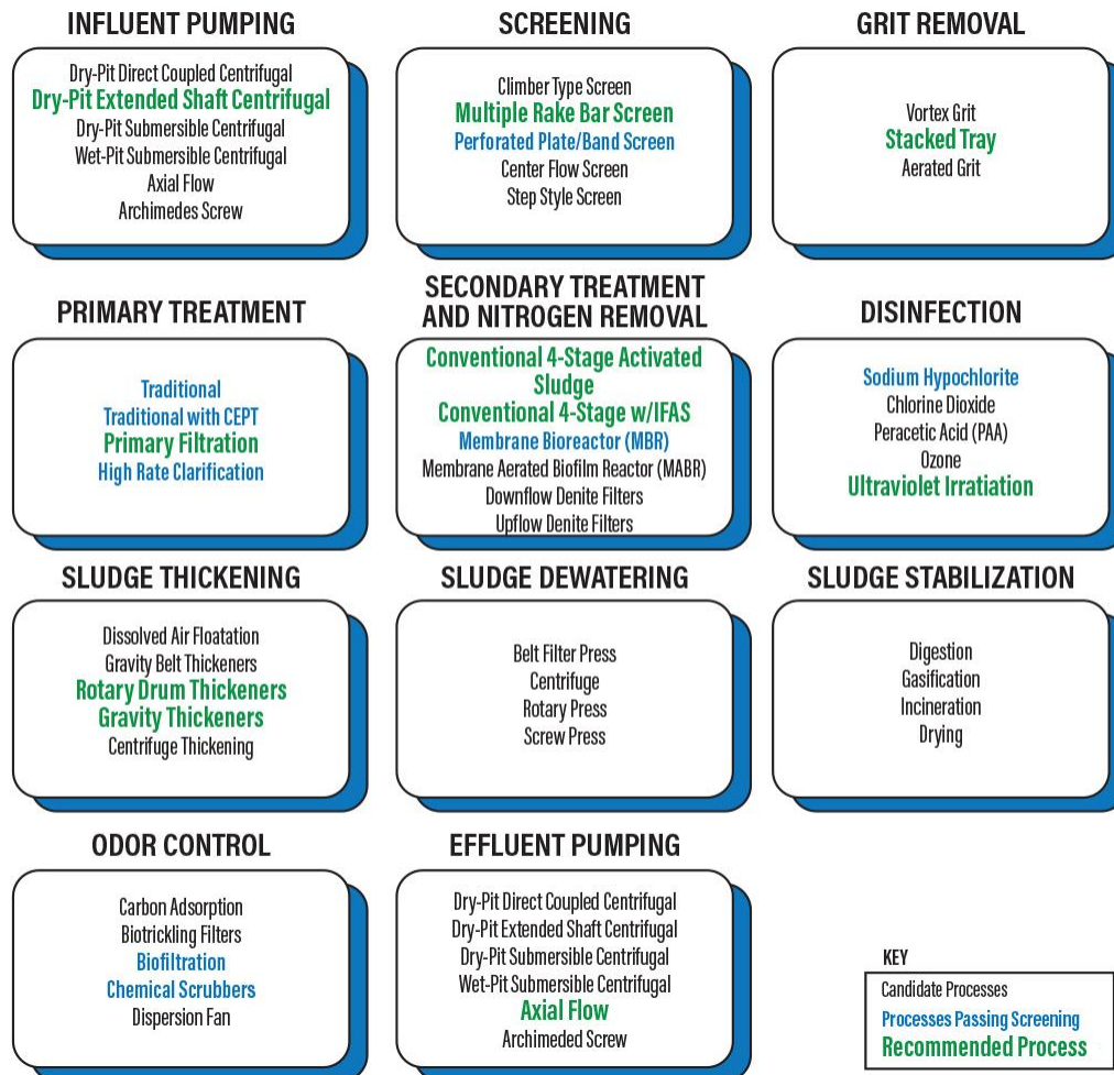
Figure ES-9 Treatment Technologies Screened and Recommended
