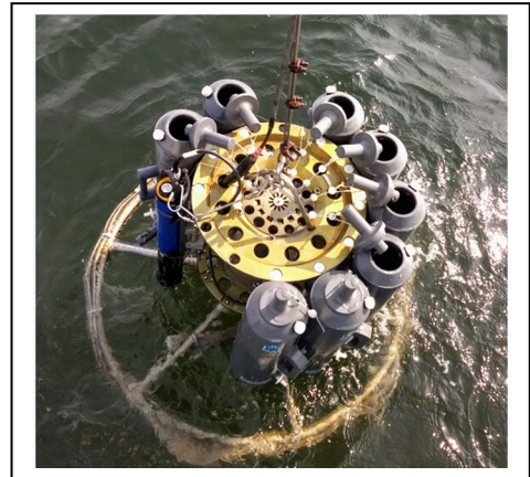
Figure 4. Rosette, profiler, and Niskin sampling array
