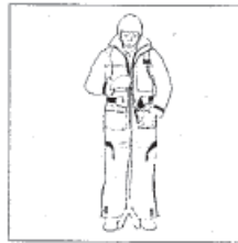
2. Close chest and leg zippers with an even pull. Secure velcro storm flap.
