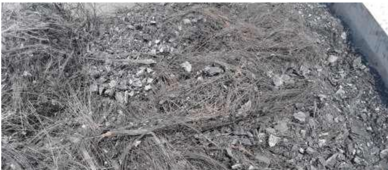
Figure 11: Char and Wire from Whole Tire Pyrolysis system. (Economics: No Shredding Equipment)
