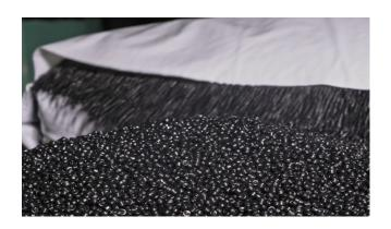
*"ELTC"* is a polymer bitumen modifier made from devulcanized crumb rubber with and without thermoplastics . ELTC is a sustainable, upcycled "Circular" material.
