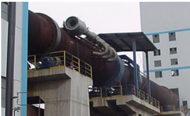
Figure 6. Metso counter current rotary kiln with mid-kiln oxidant injection
