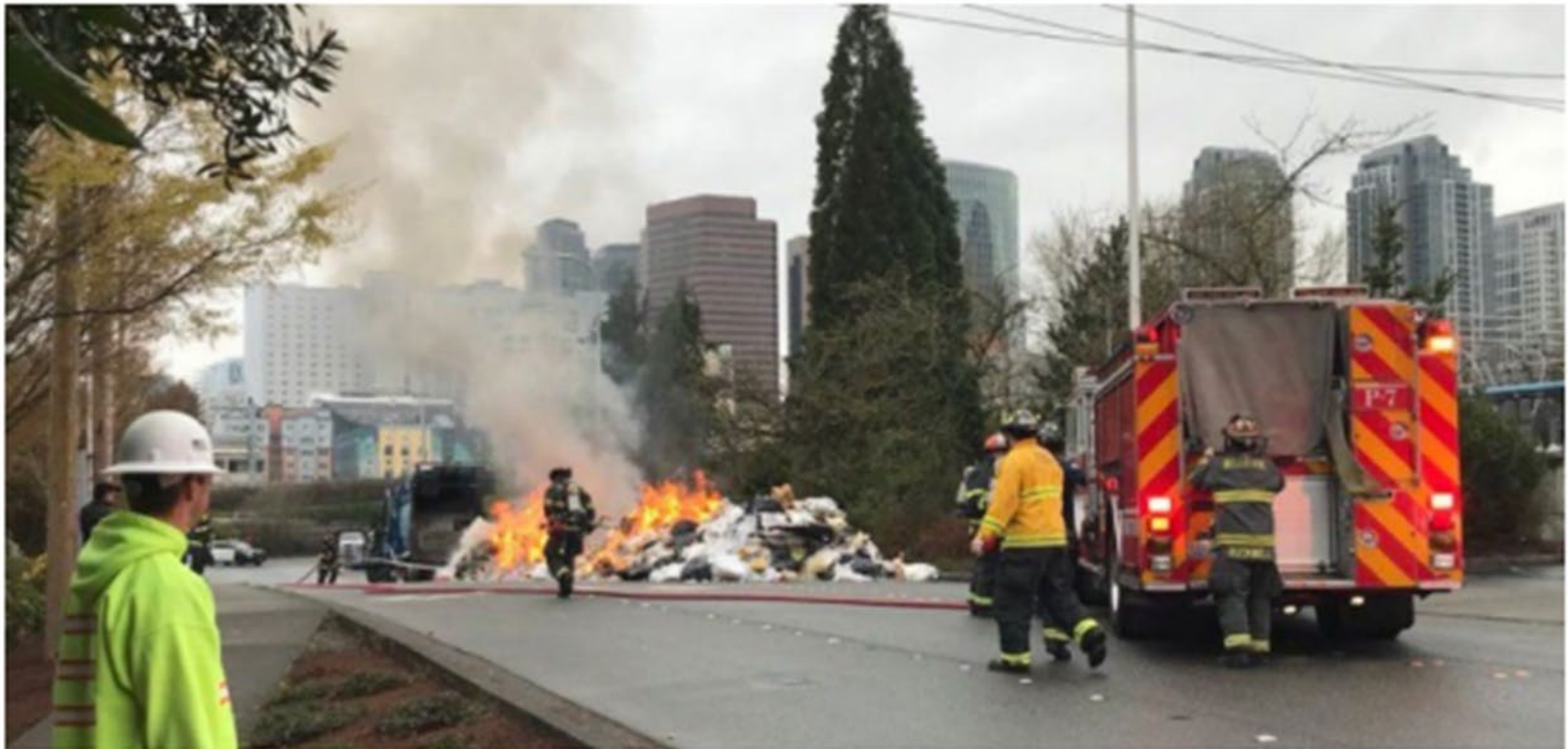
Figure 10: Photo of the aftermath of an LIB fire in a garbage truck. An LIB fire in a garbage truck forced the driver to empty garbage onto the street to be extinguished, disrupting service for customers and creating a traffic hazard for community members and first responders. Photo courtesy of Bellevue Police Department.
