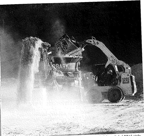
When clean drywall scrap arrives at the Marshville reclamation center, it is loaded into a Morbark 950 tub grinder.
