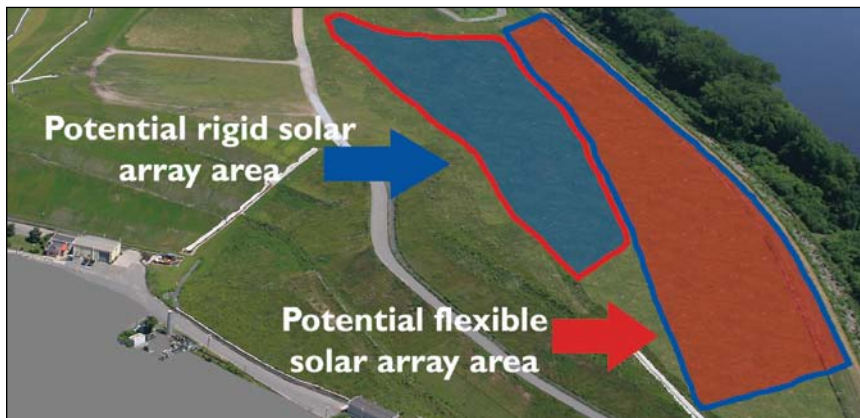
Illustration showing the areas for possible rigid or flexible solar arrays at the closed Hartford Landfill.
