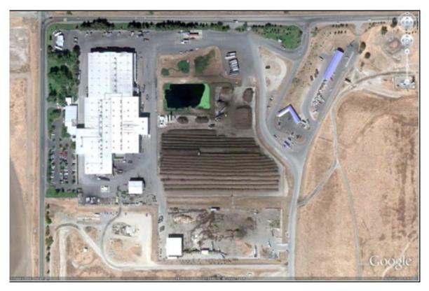
Western Placer County Integrated Facility Including Dirty MRF, Composting, C&D Processing and Landfill
