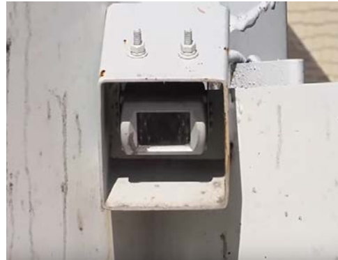
Trucks are equipped with video cameras mounted to the hopper (standard on most automated trucks)
