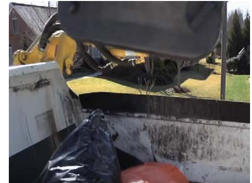
Camera clearly shows what goes into hopper – driver can easily see bags on camera inside truck
