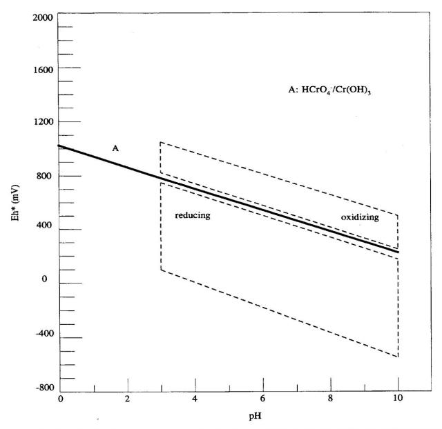
\* Note the Eh values plotted on this diagram are corrected for the reference electrode voltage: 244 mV units must be added to the measured value when a separate calomel electrode is used, or 199 mV units must be added if a combination platinum electrode is used.
