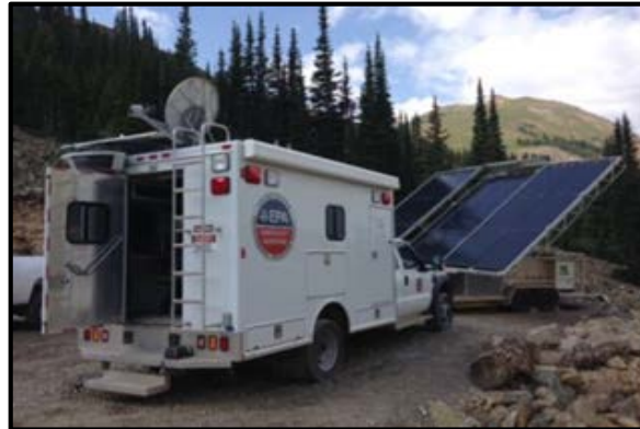
Mobile solar system to power tools
