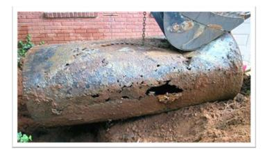
The residential home heating tanks do not have the same leak detection equipment as regulated tanks; therefore, releases are often discovered as a result of homeowners responding to the increased oil costs due to more frequent filling
