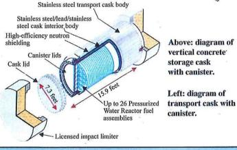
As currently planned, when the time comes to remove the SNF and GTCC waste, the dual-purpose canister will be removed from each cask, placed in an NRC licensed shipping cask, and likely transported from the site by barge or heavy haul truck. Both means of transportation were used for shipment of heavy components from the site during decommissioning.
