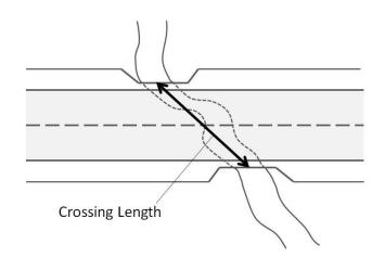
For crossing structures with multiple cells or barrels, openness is calculated separately for each cell or barrel. At least one cell or barrel must meet the appropriate openness standard. The embedded portion of a culvert is not included in the calculation of cross-sectional area for determining openness.<sup>5</sup>
