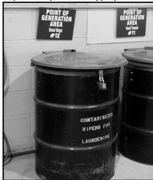
Proper storage of lint, rags & filters
