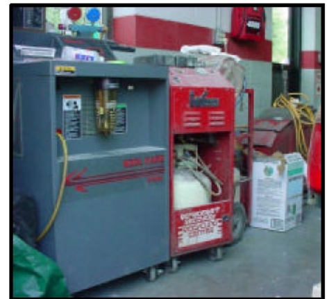
Refrigerant recovery equipment CFC-134a (left) and CFC-12 (right)
