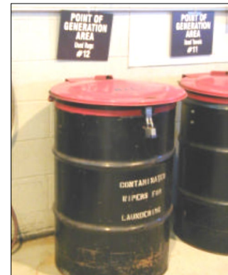
Proper storage of used rags
