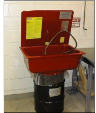
Cold Cleaning Solvent Parts Washer (Lid should be closed when not in use.)
