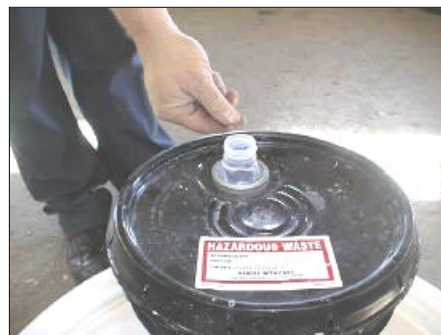
Proper storage of mercury switches
