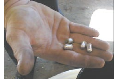
Mercury switches removed from vehicle light assemblies
