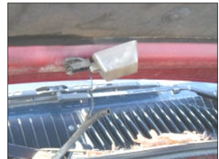
Hood light fixture with mercury switch assembly
