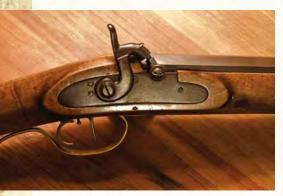
Frustrated with the relatively slow firing of the flintlock gun while duck hunting, Reverend Alexander Forsyth, a Scottish Presbyterian minister, invented the percussion cap in 1807. The percussion system uses a tiny copper or brass cup filled with a detonating compound that the shooter places on a nipple to fire the powder charge.
