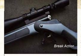
down. This exposes the breech for loading powder, attaching a cap on the nipple, cocking the hammer, and firing the gun.
