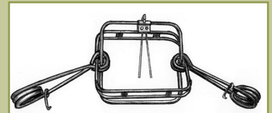
Figure FS10. Sauvageau™ bodygrip trap with additional clamping bar (set)
