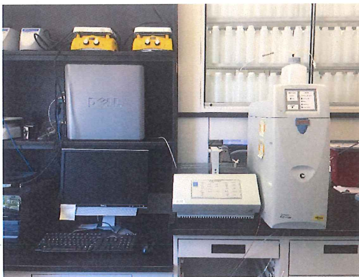
Fig. 5.7 DIONEX ICS-1100 ion chromatography
