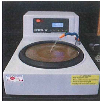
b) Rotary grinding and polishing machine
