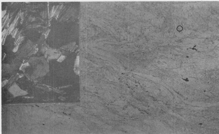
Thin section of chloritized zone of Glastonbury gneiss. Enlargement about 20X. Inset is photomicrograph of encircled area, enlargement 50X.
