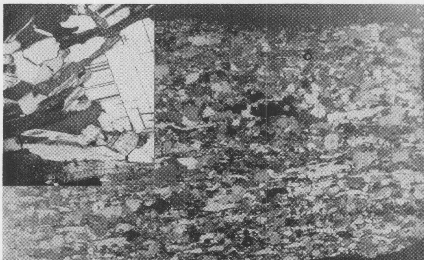
Thin section of typical Hebron gneiss. Enlargement about 20X. Inset is photomicrograph of encircled area, enlargement 50X.
