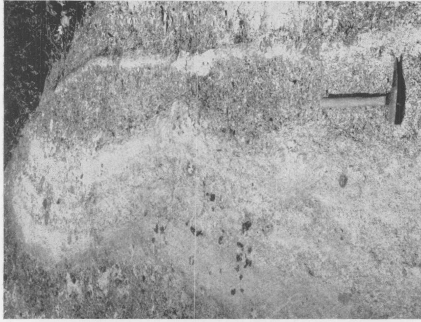
Plate III, Fig. B. Layered granite. Two fine-grained granite layers with a coarse-grained granite layer between lie to the left of the hammer. A narrow fine-grained granite layer lies to the right of the hammer. The rest of the rock in the photograph is very coarse-grained.
