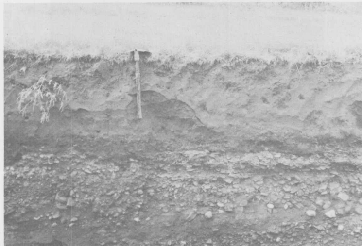
Fig. 14. Beach gravel of Lake Hitchcock overlain by 2 to 3 ft of sand. Note the angularity of the pebbles. Along West Hartford-Newington Town Line 200 ft west of South Main Street, West Hartford.
