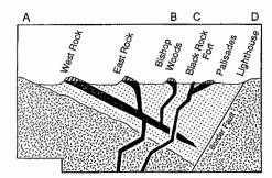
Fig. 5. Simplified geologic cross section Along line A-B-C of figure 4.
