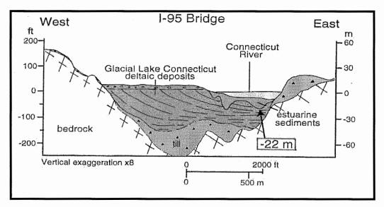
Figure 5. Geologic cross section at I-95 bridge showing the deep bedrock valley of the Connecticut River (west of the present river) filled with ice-marginal deltaic deposits, which were, in turn, incised and filled with estuarine deposits.
