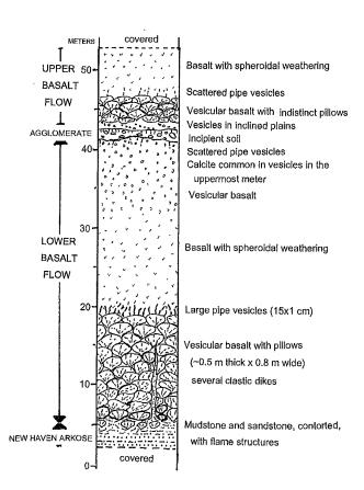
Fig. 12. Measured section of Talcott Basalt and uppermost New Haven Arkose behind Target store, Meriden
