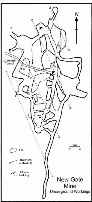
**Figure 3.** Underground workings at the New-Gate Prison mine
