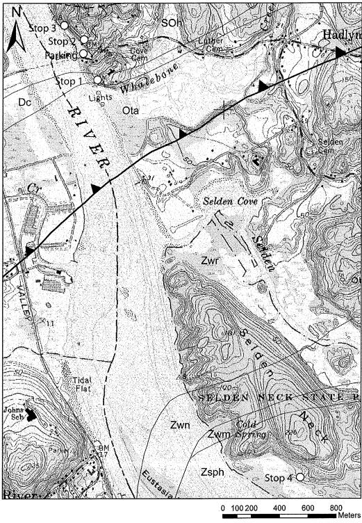
**Figure 4.** Geologic map of field trip area. Field trip stops described in text. Nashoba/Merimack/Central Maine (Iapetus) formations: Ota — Tatnic Hill Fm., Dc — Cantebury Gneiss, Soh — Hebron Gneiss; Avalonian terrane formations: Zw — Waterford Group, Zwn — New London Gneiss, Zwm — Mamacoke Fm., Zsph — Potter Hill Granite Gneiss. Honey Hill fault is toothed bold line separating Ota from Zwr. Geology from Rogers (1985). USGS Topo base.
