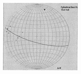
**Figure 5.** Equal area plot of foliation from Stop 1. Great circle is cylindrical best fit to data.
