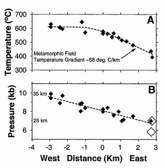
Figure 2. Estimates of metamorphic temperatures and pressures across the Wepawaug Schist. Modified after Ague (2002).
