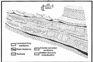
Figure 4. Schematic cross-section of the ore bed at New-Gate
