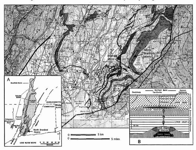
Figure 1. Geological map of the southeastern part of the Hartford Basin (from Rodgers, 1985) and location of the North Branford quarry. Inset A shows the distribution of the three volcanic units in the Hartford Basin – Talcott, Holyoke, and Hampden—and their associated dikes (Higganum, Buttress, and Bridgeport) and sills. Inset B shows a hypothetical cross section across the Hartford Basin at the time of the Holyoke eruption (Philpotts, 1998).
