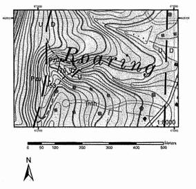
Figure 5. Left: Sketch map of the Western Border Fault in Southington. Box shows location of close-up map. Right: close-up map of stop 1. Pzu – undifferentiated Paleozoic, Trnh – Triassic New Haven Formation. Modified from Fritts (1963).
