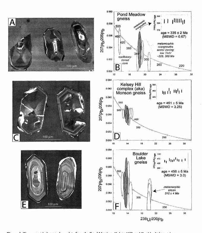
Figure 6. Zircon morphology and age data from the Pond Meadow, Kelsey Hill, and Boulder Lake gneisses. The oscillatory zoning in cores of zircons from the Kelsey Hill and Boulder Lake gneisses indicates crystallization in a magma, whereas sector zoning in broad mantles of zircons from the Pond Meadow gneiss suggests growth during metamorphism.
