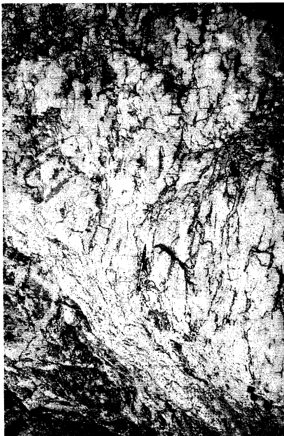
Figure 24. Joints cutting massive quartz of the Lantern Hill quartz lode, North Stonington, Connecticut. Note the curvature or change in orientation of joints in proximity to a dense zone of fractures. Curved joints may record evidence of stress perturbation in proximity to a fracture zone.
