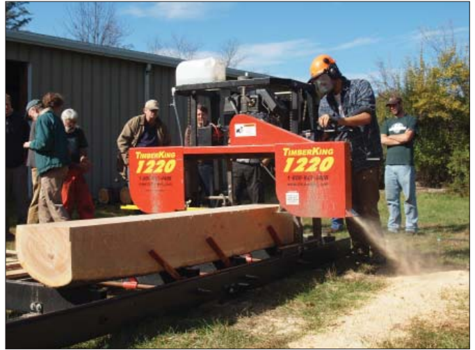
Portable sawmill in action, as part of same workshop. The log being milled was a high value cherry log harvested on the grounds.
