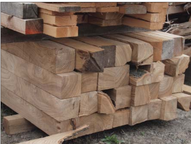
Black locust cants in a lumber mill. Black locust is relatively uncommon commercially but is very useful due to its natural decay resistance.
