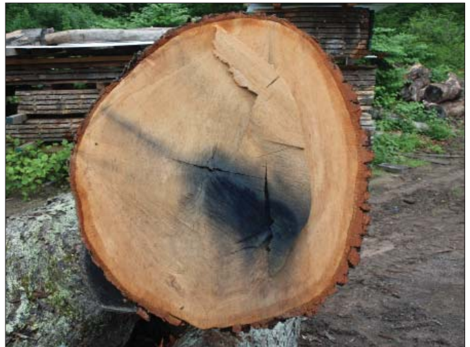
Blue-black staining on an oak log, indicating the presence of iron within that log. The sawyer will be careful to avoid this metal if possible.
