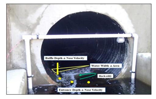
*Figure 15. Collection of hydraulic condition data at 1<sup>st</sup> baffle and culvert entrance in 2017.*
