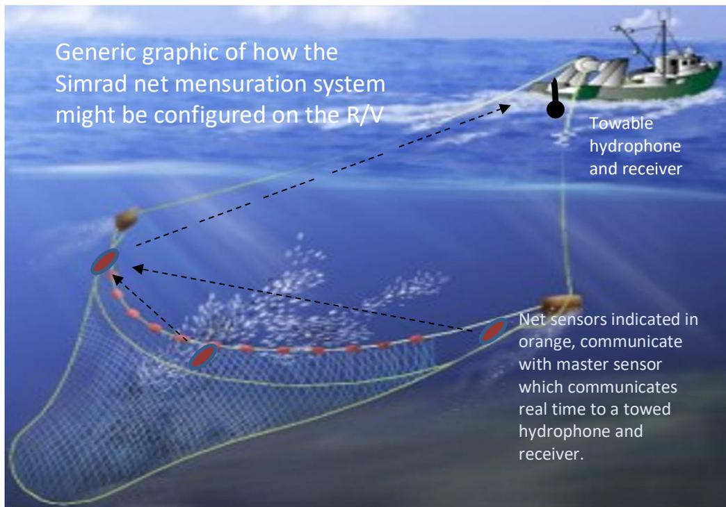
Schematic of how the components of the Simrad net mensuration system might be situated on the R/V John Dempsey and net.
