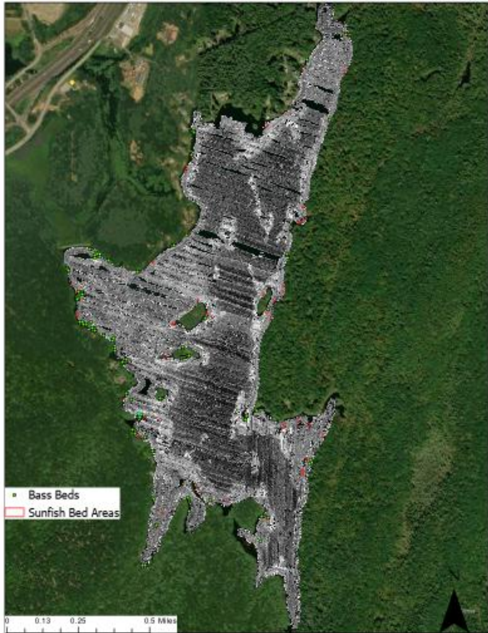
Figure 8. Georeferenced Side Scan Sonar Imagery and Centrarchid Bed Locations for Mashapaug Lake.
