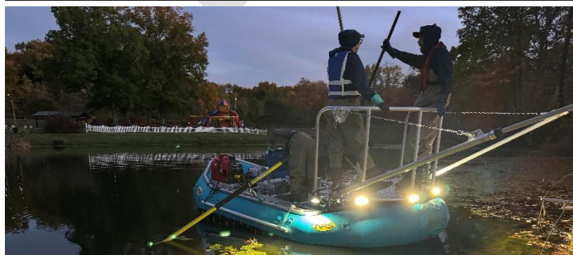
A crew preparing to night sample a Community Fishing Water. The new FD electrofishing raft allows us to adaptively manage many waterbodies that were previously inaccessible to our sampling gear.
