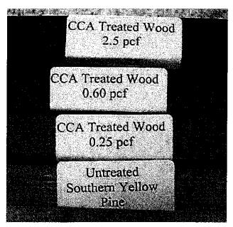
The photo at the left is from the above referenced Florida report, and illustrates the gradations in coloring for treated wood, compared to untreated wood. Regulated Wood Fuel Producers are to train their staff in the visual identification of treated wood.
