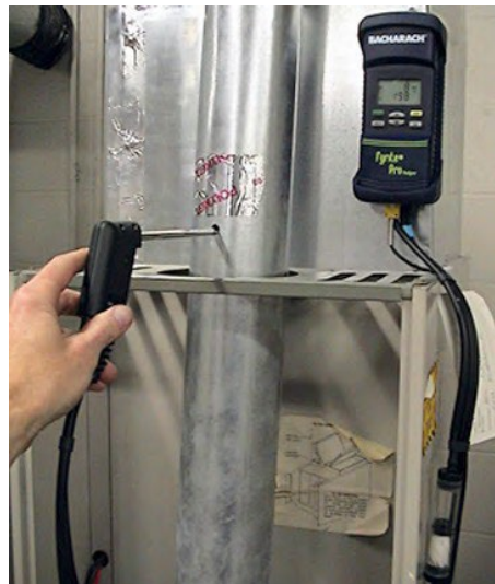
80+ Furnace: Measure draft and sample flue gases in the vent connector above the furnace.
