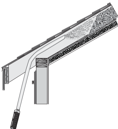
Blowing from the eaves: Some vaulted ceilings can be blown from the eaves and/ or the ridge.
