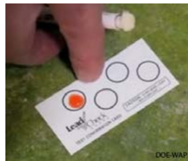
If the surface tests negative, verify the validity of the test with the calibration card provided.
