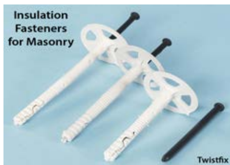
Rigid-foam fasteners for masonry: Installers use power drivers to fasten rigid foam to masonry materials.
