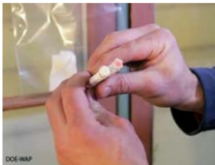
Red means lead-positive and white means lead-negative.
