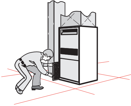
Panel filter installed in filter slot in return plenum
