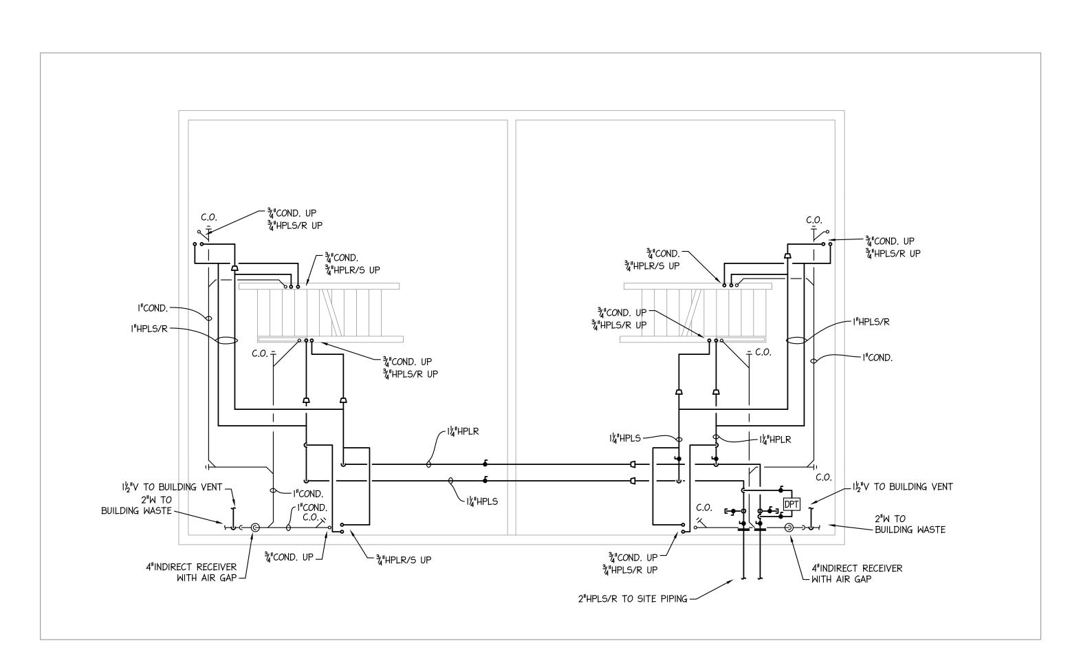
1) TYP. 2-UNIT TYPE A MECH./PLUMB. NEW WORK PLAN - BASEMENT
