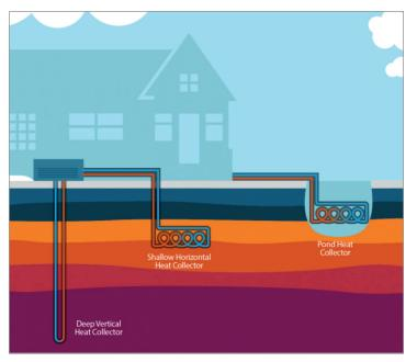
Figure 1. Adapted from the <u>U.S. Department of Energy</u> showing configurations of ground loops
