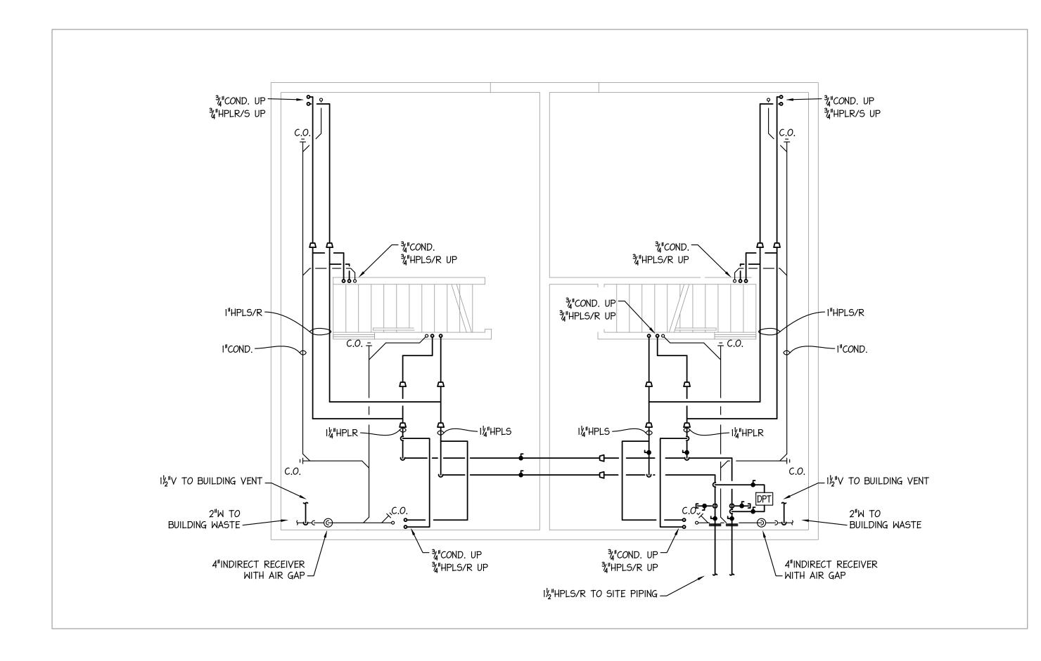
1) TYP. 2-UNIT TYPE B MECH./PLUMB. NEW WORK PLAN - BASEMENT
