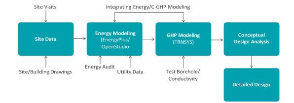
Figure 4. Schematic of the community geothermal heat pump system modeling and design process.
