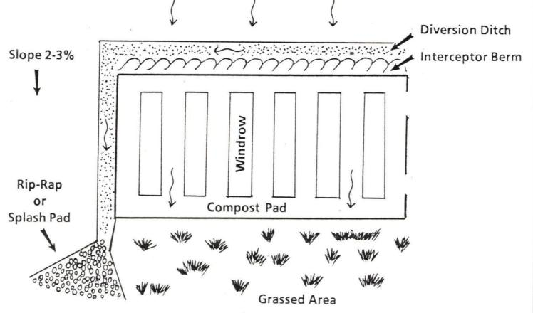
Generic Site Plan to Control Run-off and Run-on
