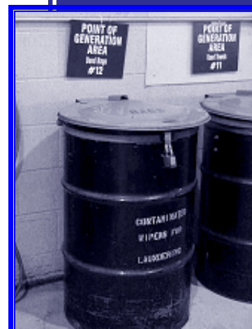
Proper storage of used rags
