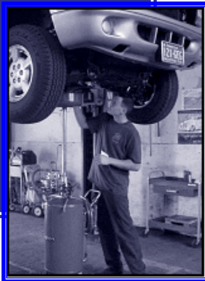
Vacuum-type drain system
