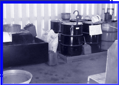
Container storage area with containment.
